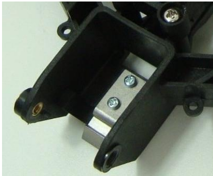
Check the (6) Arm Latch/catch screws tight.
