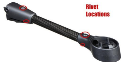
Arm - lightly twist and check rivets secure
