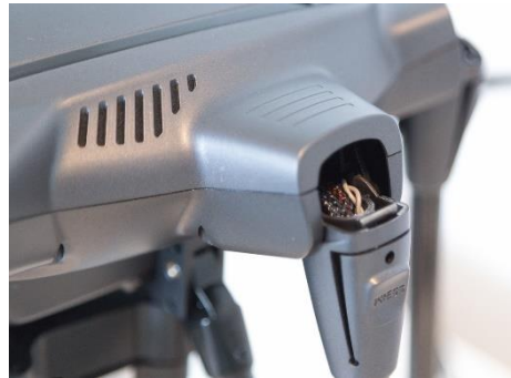
Inspect motor wire protective sleeve.
