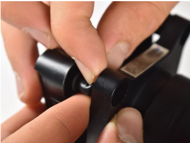
To Help push these dampeners back into place, use a blunt skinny tool. While holding the two plates together.
