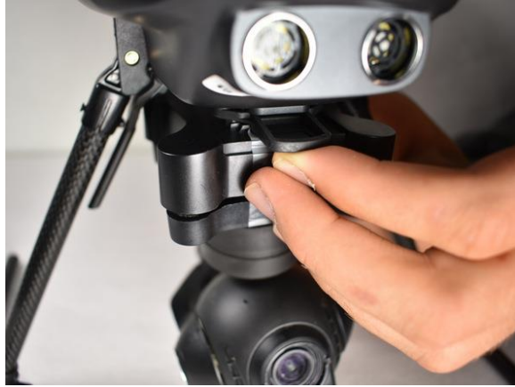
Push up on the tab connected to the camera configuration and slide the entire apparatus off.
