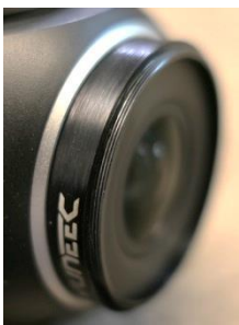
Check the threads for damage
