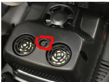
Cooling Fan, Sonar, Pin Camera (red)
