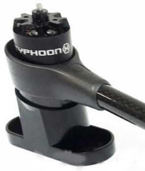
Twist tool to remove Lens
