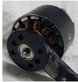
Bottom of motor with C clip & washer removed
