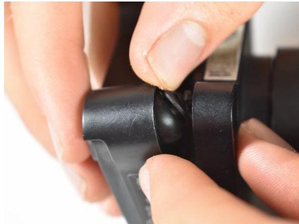
Put the gimbal damper (the rubber balls) back into the plastic alignment mounts.
